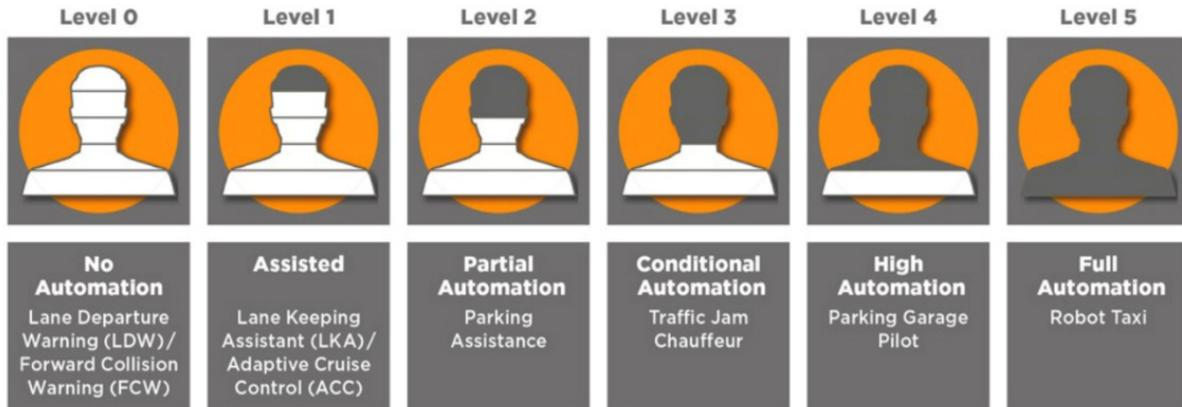
The levels of vehicle automation according to the Society of Automotive Engineers (SAE) 2018.
